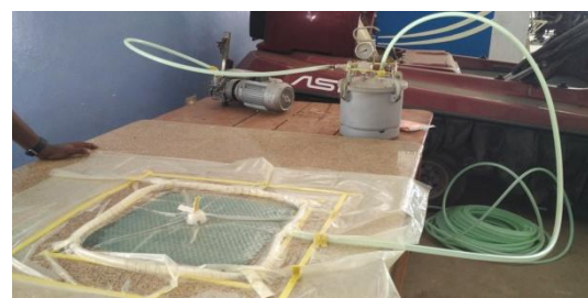
Figure 5-Original setup of vacuum infusion process Cutting of test specimens
